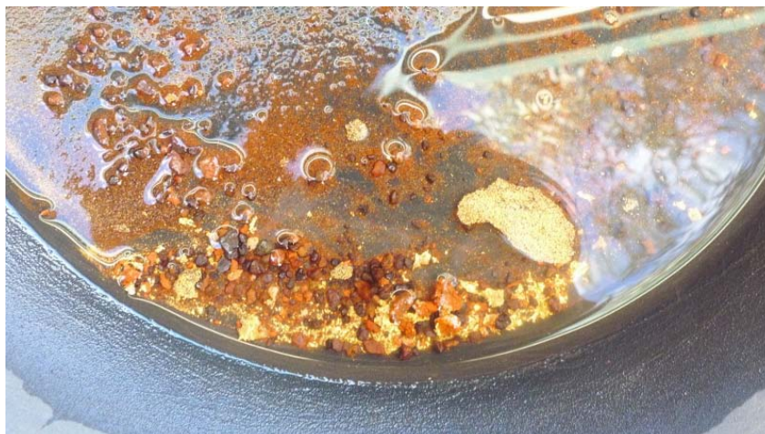
Figure 2: Free gold panned from Koopman's Find patch at Tobin Hill area. Note floating fine gold
