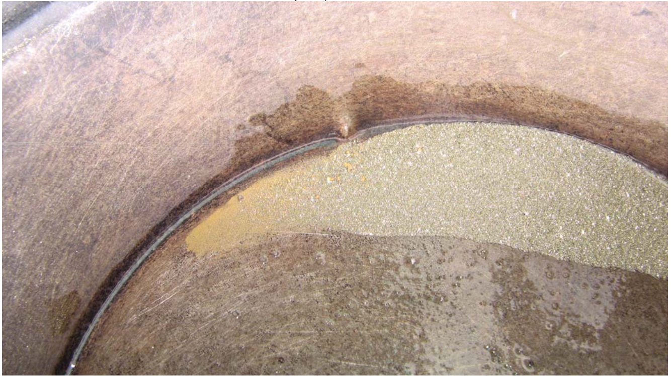
Figure 2: Photo Showing a Tail of Free Gold Panned from 226-227m Intercept in Hole 10EYRC0103 (Fine Yellow Gold and Silvery Sulphides).
