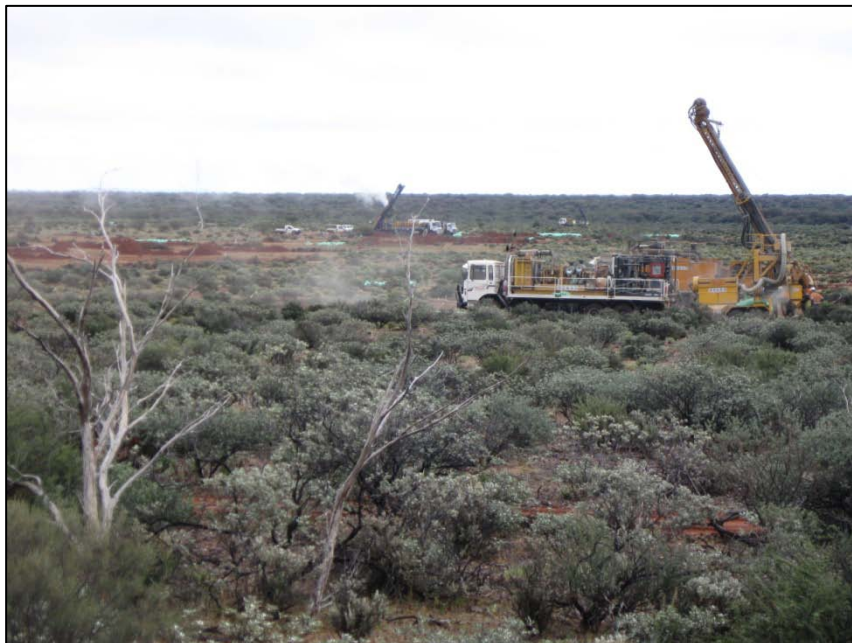
Figure 3: Photo showing all three rigs (2 RC and 1 RAB) in close proximity actively drilling at Central Bore and Justinian projects.
