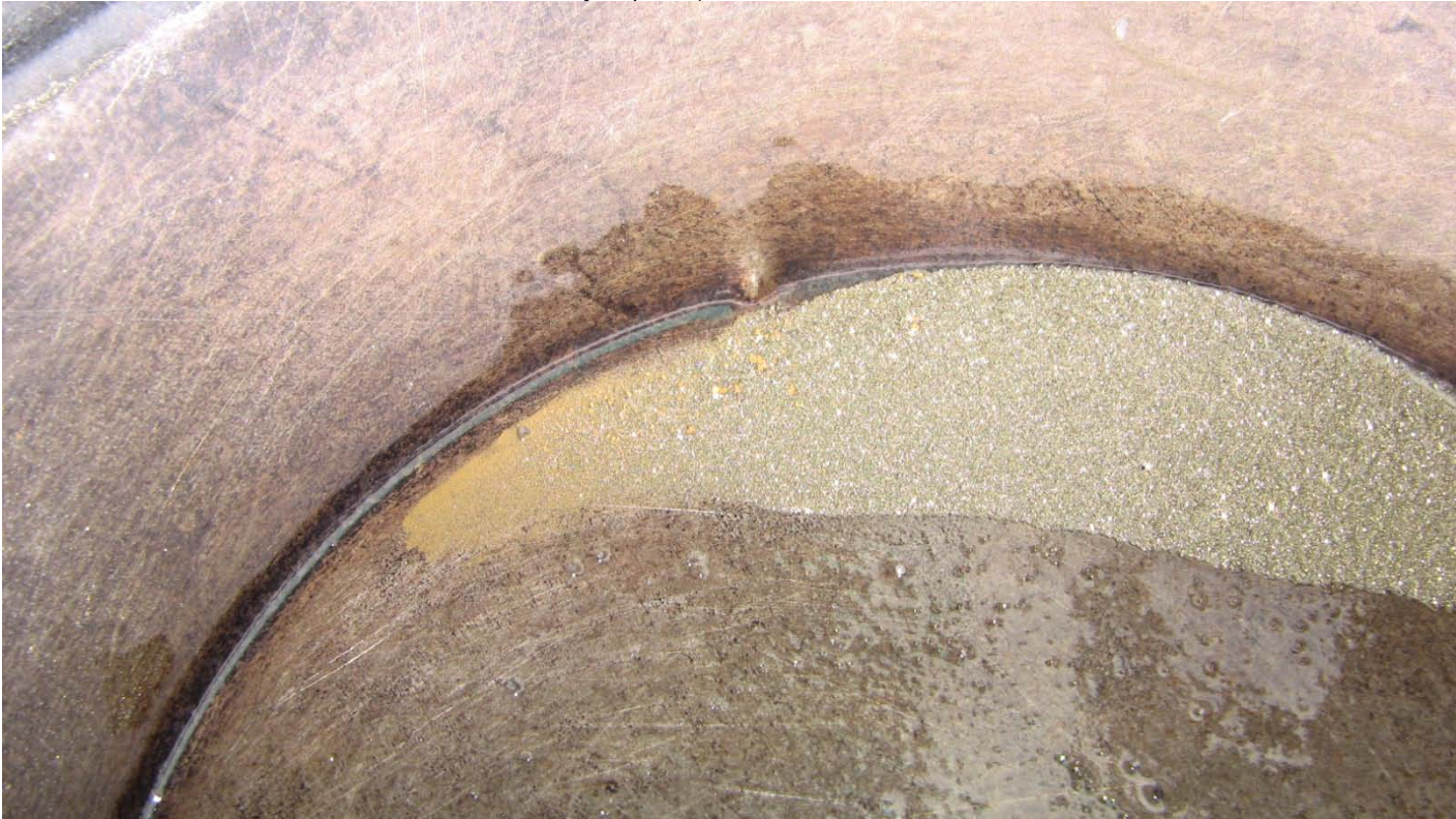
Figure 3: Photo Showing a Tail of Free Gold Panned from 226-227m Intercept in Hole 10EYRC0103 (Fine Yellow Gold and Silvery Sulphides).
