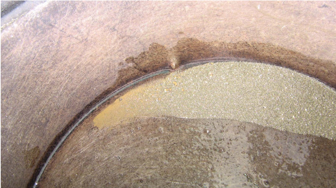
Figure 8: Photo Showing a Tail of Free Gold Panned from 226-227m Intercept in Hole 10EYRC0103 (Fine Yellow Gold and Silvery Sulphides).
